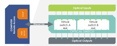
For example, virtual switch A rate is 1,0625 Gbps and virtual switch B rate is 3,1875 Gbps
